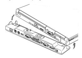
Figure 4-14 Attaching the Port Replicator
